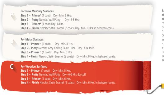
Sand the surface with Emery Paper and wipe clean before application on subsequent coats.
